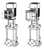
2. Fix the machine on the bottom plate, remove the wiring surface shell on the right side of the machine, so that the pump output line, the input line of the frequency converter and the sensor line pass through the waterproof joint successively, and fix it according to the mark.
